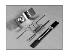
Special Boat for aperture cleaning will hold several apertures at one time
