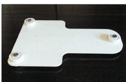
Underside of Platform showing Isolators
