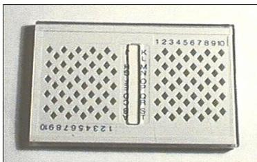
These boxes hold up to 100 grids in numbered holes, designed to take either 3.05mm or 2.3mm grids accessed a row at a time through a slot in the sliding cover. Dimensions; 85 x 58 x 7mm high. Complete with grid recording card.
