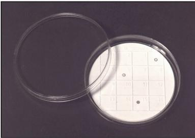
Round silicone rubber indexed grid storage plate numbered. Available in two sizes 85mm and 45mm diameter which are supplied mounted in either 90mm or 50mm plastic Petri dish or supplied loose. This is an ideal way of storing "working grids" or staining grids. The grids adhere lightly to the silicone plate, which eliminates the problem of grids jumping. The grids are easily picked up without damaging the tweezer tips or the grid.
