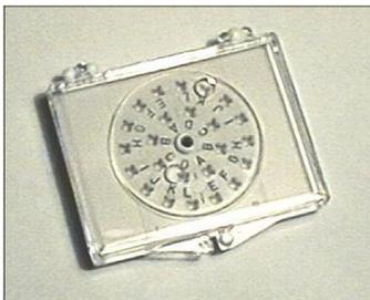
Indexed grid box containing 24 letter-labelled crossed slots, which accommodate 3.05mm in one direction and 2.3mm in the other. The grids are accessed one at a time through a hole in the clear rotating protection disc. The box is totally enclosed by a hinged lid making the box fully dust proof.
