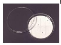
Round silicone rubber indexed grid storage plate numbered. Available in two sizes 85mm and 45mm diameter which are supplied mounted in either 90mm or 50mm plastic Petri dish or supplied loose. This is an ideal way of storing "working grids" or staining grids. The grids adhere lightly to the silicone plate, which eliminates the problem of grids jumping. The grids are easily picked up without damaging the tweezer tips or the grid.
