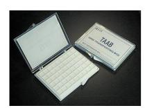
Designed to store or transport grids this TAAB box has an indexed silicone rubber plate housed in a transparent viewing box with hinged lid.
