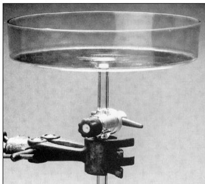
Settlement dish, 135mm diameter with drain tap. Useful for removing distilled water when preparing formvar, butvar or collodion support films, or for floating down stripped carbon films on to TEM grids.
