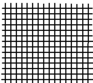
A fine but rigid stainless steel mesh 150 x 150mm square with a mesh size of approximately 0.5mm that can be used with the settlement dish as a support to receive the grids after they are placed on the support film.
