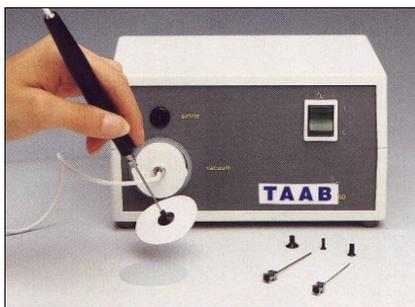
Useful for handling without damage, small, delicate items i.e. grids, specimens etc. The suction can be applied through a selection of either fine tubes or rubber suckers actuated by covering the hole in the tube with a finger. The object being lifted is released by lifting the finger from the hole. Nozzle sizes are 0.4mm, 0.7mm and 1.0mm.
