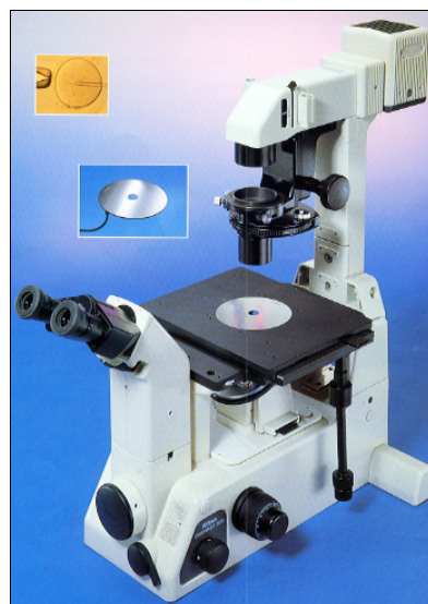
Bio Cryo Stage BCS 196 -196° to 125°C
