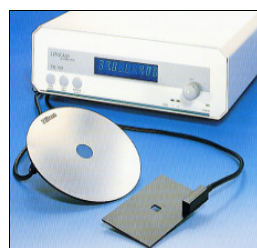
C102 Controller with two of several warm stages
