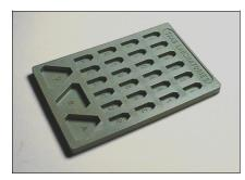
This green silicone rubber mould has **24** self numbered cavities and produces blocks with trapezoidal tip at one end for easy trimming. The produced block is 14mm x 6mm x 4mm deep and the mould also contains **3** special cavities for multiple embedding which can hold **3** samples in each cavity. Overall size of mould 118mm x 78mm.
