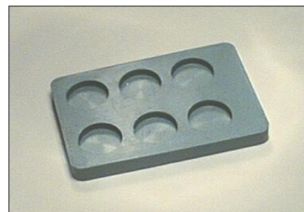
Block Holder S264 shown holding flat resin block See page 5.19 for more details.
