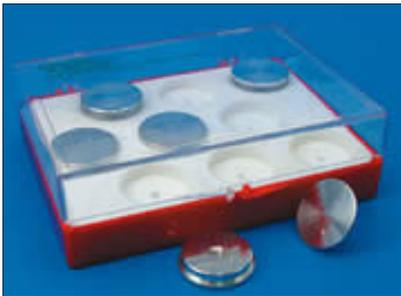
This box accommodates up to **9 mounting stubs** of either 1" (25mm) in diameter or a stub with 1/8" (3.2mm) diameter pin.
