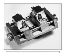
The thumbwheel clamp has single operation symmetrical vice motion with reversible clamping bars to give different sized indentations to clamp irregular shaped specimens. Two models are available for specimens up to 34mm or up to 51mm
