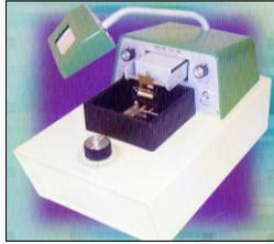
The Vibratome 1000 is the original vibrating tissue sectioning system and provides semi-automatic sectioning with simple precise controls and adjustments for cutting fresh or fixed tissue down to 20µm thickness. It is quiet in operation, has click stops at 10µm intervals, height and tilt adjustments, stable blade holder and a cool lamp magnifier.
