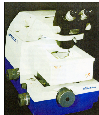
CR-X attached to Ultracut ultramicrotome
