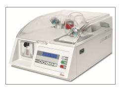
The Leica EM AC20 automatic contrasting system for ultrathin sections ensures minimum user contact with reagents and reduced reagent consumption staining up to 20 grids per run. Use of a peristaltic pump and non-contact valves allow the reagents to travel directly through tubing to the grid chamber, resulting in fast, high-quality double staining and easy maintenance.
