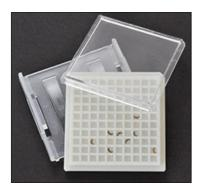
**Storage box to hold 100 Omniprobe** half grids or standard 3mm  $\varnothing$  TEM grids flat. No adhesive in tray (made from ABS). Cavity size is 3.34 x 3.34 x 1.5mm (0.13" x 0.13" x 0.06"). Complete with clear polystyrene lid and clear polypropylene clip. Stackable. Overall size is 55 x 51 x 10.7mm (2.16" x 2" x 0.42")
