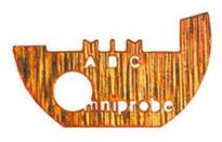
**3 post** lift-out grids  $3mm \, \mathcal{O}$ ,  $35\mu m$  thick with 1 edge lower for easy access. These grids include multiple indexed mounting locations, two with vertical bar attachment surfaces and two with "V" shaped alignment surfaces. Packaged in glass vials.
