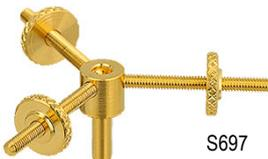
**Lightweight, spider like holder** for awkwardly shaped samples up to 45mm Ø. Samples are supported by the three threaded legs and clamped by the flanges on the clamping nuts. Made from brass and plated with 1µm of pure gold.
