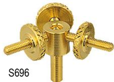
**Lightweight, spider like holder** for awkwardly shaped samples up to 25mm Ø. Samples are supported by the three threaded legs and clamped by the flanges on the clamping nuts. Made from brass and plated with 1µm of pure gold.
