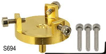
**Round type bulk sample holder** with three brackets for round and awkwardly shaped samples up to 20mm Ø. Made from brass, 1µm thick gold plated. Ideal for smaller samples and smaller SEMs. Provided with 6 set screws.
