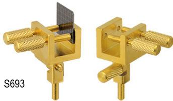
**A swivel vice which covers a full 180° angle** and can also be rotated with the stub. This is the ultimate holder for imaging cross sections at any desired angle. The swivel head size without clamping screws is only 16 x16 x 14mm. The sample is clamped with the two knurled clamping screws; the swivel head can be locked in place with the tilt clamping screw. Made from brass and plated with 1µm of pure gold.
