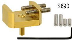
**Rectangular type bulk sample holder** with pin (or M4) and two side brackets for sample thickness up to 16mm. Made from brass, 1µm thick gold plated. Ideal for smaller samples and smaller SEMs. Provided with 4 set screws.
