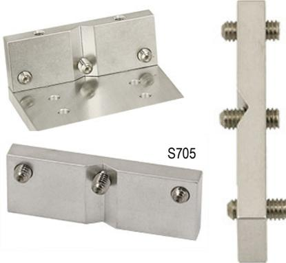
The grooved vice clamping plates can be mounted either way to optimise the height of the clamping screws. When the grooved vice clamping plates are attached in the standard position, the clamping screws are in a higher position. Attach the grooved clamping plates upside down and the clamping screw will be in a lower position.
