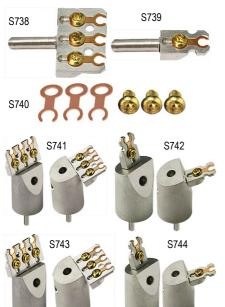
\$738 t-EBSD holder for three (3) TEM/FIB lift-out grids standard pin
