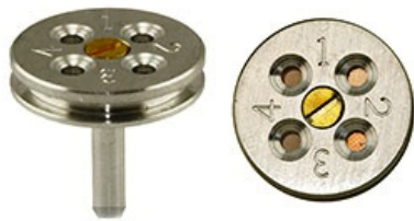
S400 TG4 TEM grid holder securely holds up to 4x TEM grids, 18 x 3.2mm Ø, aluminium, pin base
