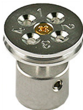
S795 TG4J TEM grid holder securely holds up to 4 TEM grids, 18 x 3.2mm Ø, aluminium, pin base with JEOL 12.2mm Ø stub adaptor
