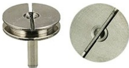
S793 PS11 mini TEM grid holder securely holds 1x TEM grid, 12.7 x 3.2mm Ø, aluminium, pin base
