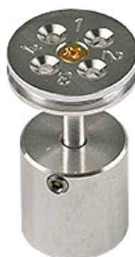
S401 TG4C TEM grid holder securely holds up to 4x TEM grids, 18 x 3.2mm Ø, copper, pin base
