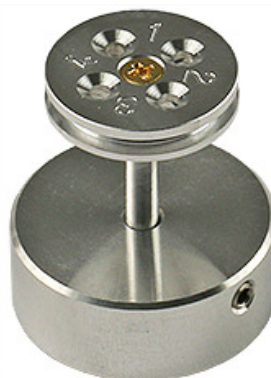
S795 TG4J TEM grid holder securely holds up to 4 TEM grids, 18 x 3.2mm Ø, aluminium, pin base with JEOL 12.2mm Ø stub adaptor
