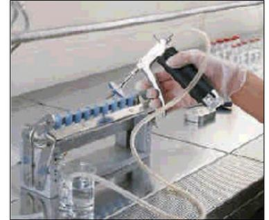
Minisart-plus units are of advantage for the sterilisation of difficult to filter liquids. They include a fine glass fibre prefilter on the membrane filter, a combination which is so effective that throughputs can often be doubled. Minisarts and their packaging are environmentally friendly, free of PVC.
