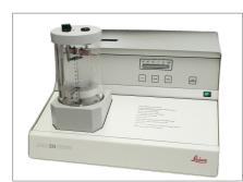
A **compact bench-top** single and multiple carbon thread evaporator producing conductive carbon films on specimens for X-ray microanalysis (EDX, WDX) and carbon reinforcement films on collodion or formvar coated specimen support grids for TEM. Uses flash or pulsation evaporation under low vacuum vacuum conditions. Carbon thread produces cohesive films that will cover very fissured surfaces.
